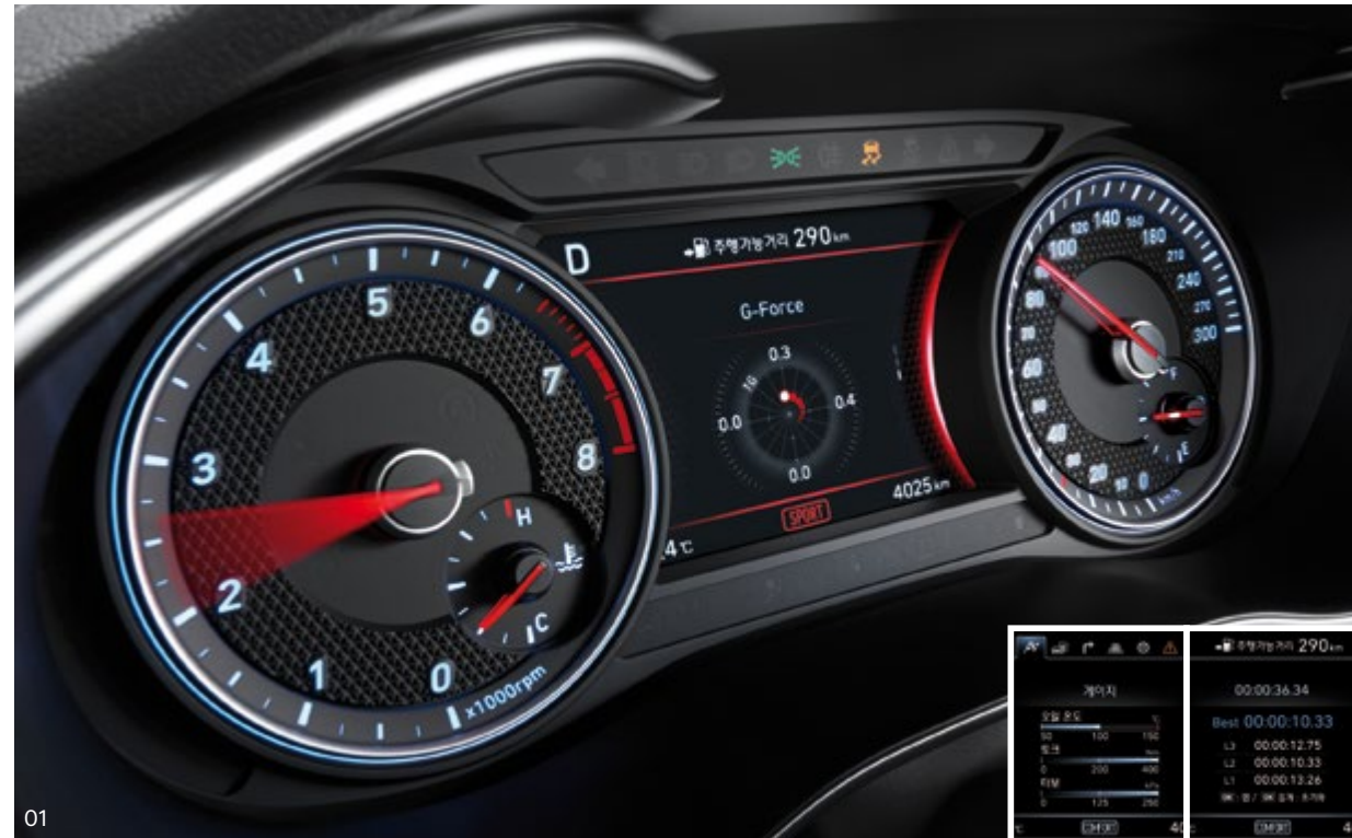
01. 7" TFT LCD cluster _ The engine oil temperature gauge, torque gauge, turbo booster gauge, lap timer (shows the best and the 3 most recent lap times), and G-Force (shows the current top, bottom, left, and right gravity acceleration or G values) can be seen through the cluster which also amplifies the enjoyment of high-performance driving with differentiated content.
