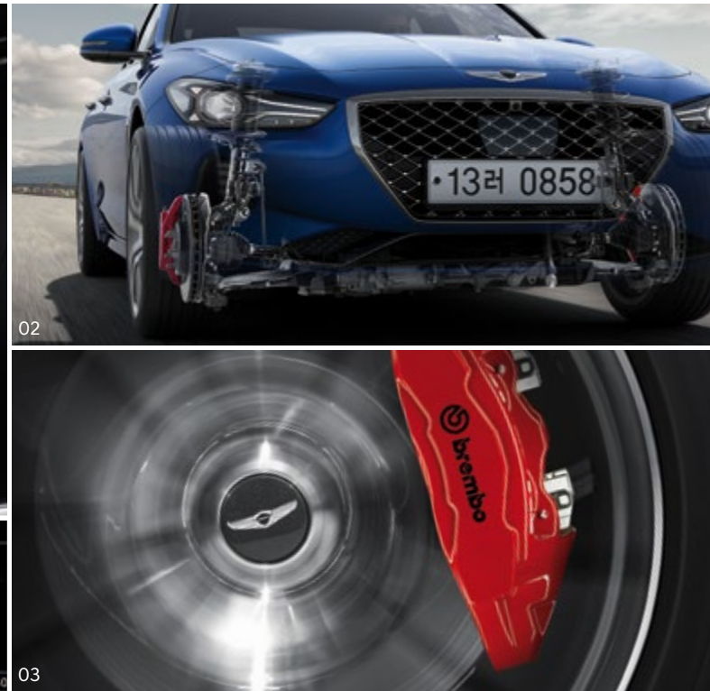
02. Sports suspension (Electronic control) _ Driving stability and ride comfort are achieved simultaneously with shock absorbers that adjust damping force according to road surface and driving conditions. The use of aluminum on the sports suspension (electronic control) and the lower arm of the amplitude-sensitive damper suspension reduces weight. 03. Brembo brakes _ To deliver the differentiated image and overpowering driving performance of a high-performance sports sedan, 3.3T Sport is equipped with Brembo brakes, offering superior quality and braking performance.
